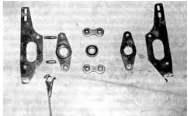
FIGURE 4. Failed Knife Drive Mechanism.
