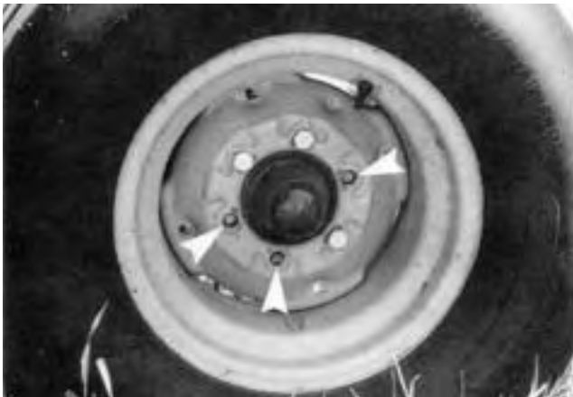
FIGURE 4. Broken Wheel Bolts.
