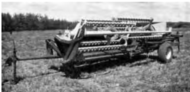
FIGURE 6. Full Transport Position.
