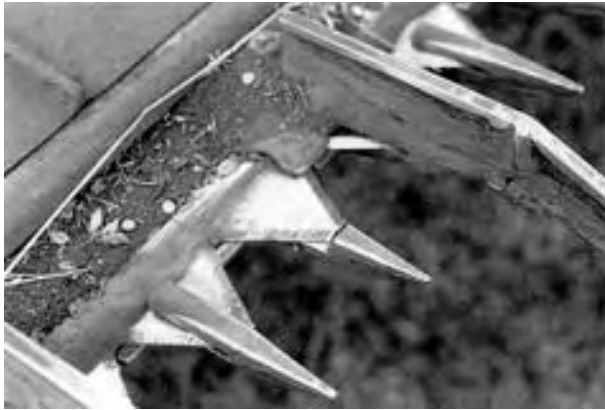
FIGURE 2. Crop Material Adhesion and Buildup.
