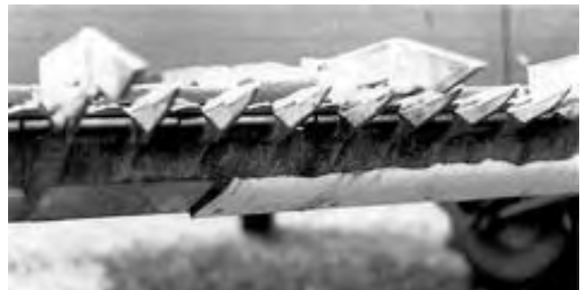
FIGURE 11. Adhesion on Both Steel and Polyethylene in Wet Weedy Conditions.
