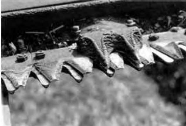
FIGURE 6. Crop Material Adhesion and Buildup.
