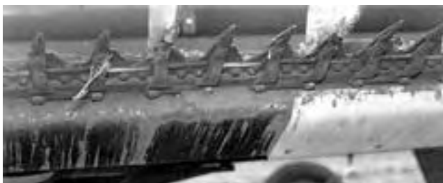
FIGURE 10. Adhesion to Steel only in Moist Conditions.
