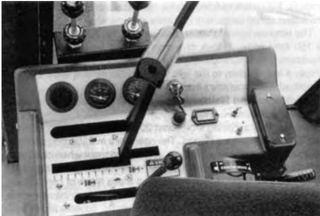
FIGURE 11. Operator Station Instruments and Controls.
