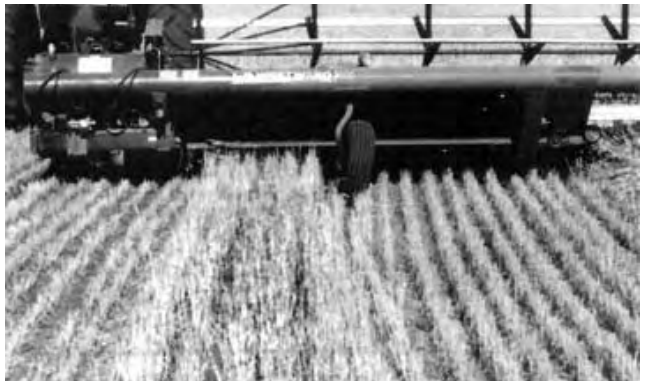
FIGURE 4. Barrier Strip Formation and Position.
