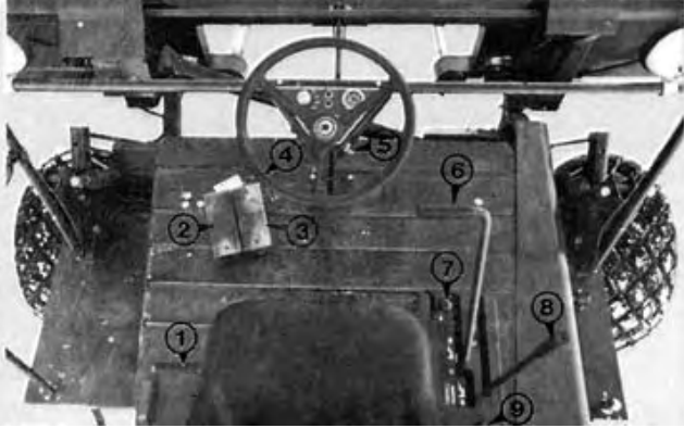
FIGURE 1. Operator's Platform. 1) Parking Brake Lever, 2) Reel Hydraulic Control Pedal, 3) Header Hydraulic Control Pedal, 4) Steering Wheel, 5) Ignition Switch, 6) Speed Control Lever, 7) Throttle, 8) Header Control Lever, 9) Choke.
