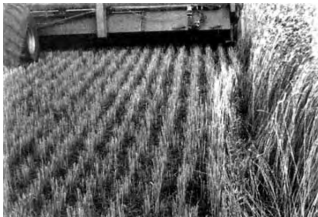
FIGURE 2. Crop Flattened by the Optional Gauge Wheel.
