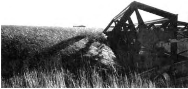
FIGURE 3. Inadequate Forward Reel Positioning.
