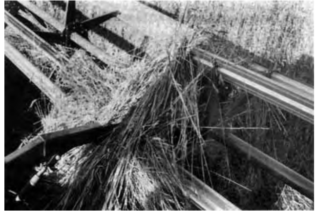
FIGURE 2. Material Caught on the Reel Arm.
