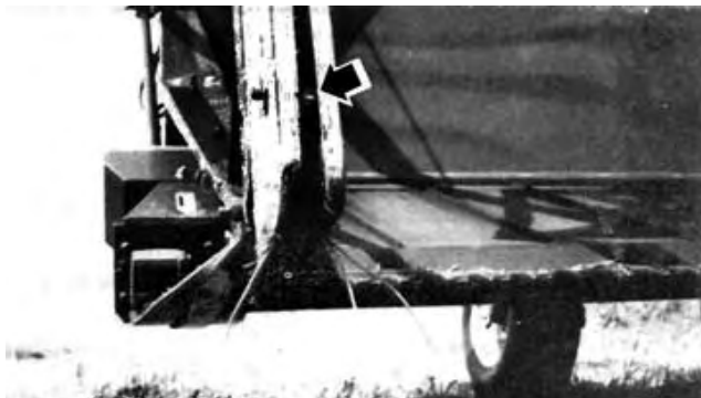
FIGURE 4. Keer Shear Stopped by Small Stone.
