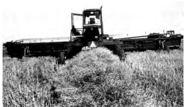
FIGURE 1. Windrowing Rapeseed with the Keer Shear Attachment.
