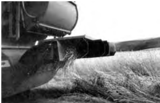
FIGURE 3. Tough Wheat Straw Wedged Between Fourth and Fifth Distribution Vanes.
