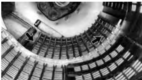
FIGURE 19. Damaged Hardened Surface and Bent Concave Bars.
