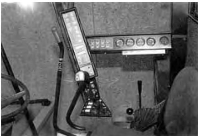
FIGURE 17. Instrument and Control Console.
