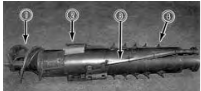
FIGURE 2. "S" Cubed Rotor: (1) Intake Flighting and Wear Plate, (2) Rasp Bars, (3) Separating Blades, (4) Agitating Pins.
