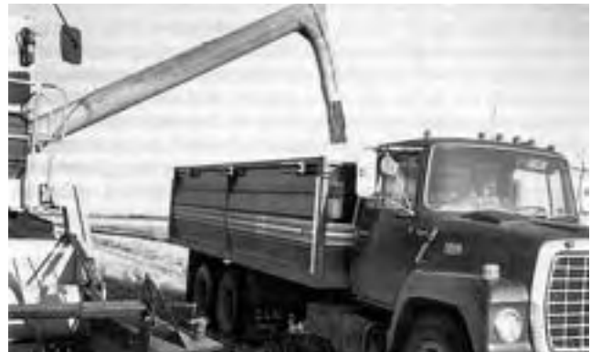
FIGURE 14. PAMI Installed Loading Spout.
