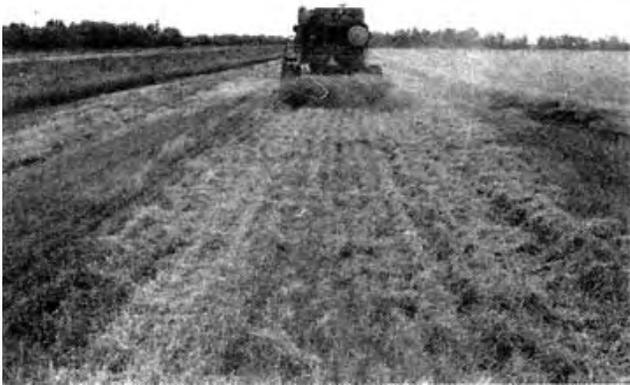
FIGURE 15. Typical Straw Spread Pattern.
