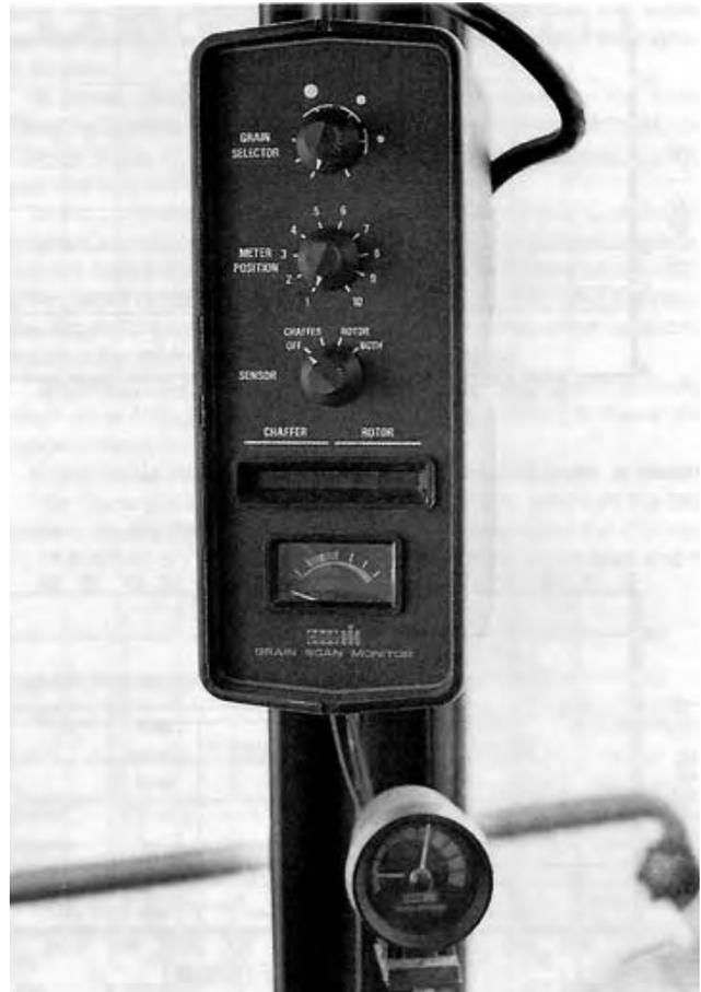
FIGURE 18. Loss Monitor Console.
