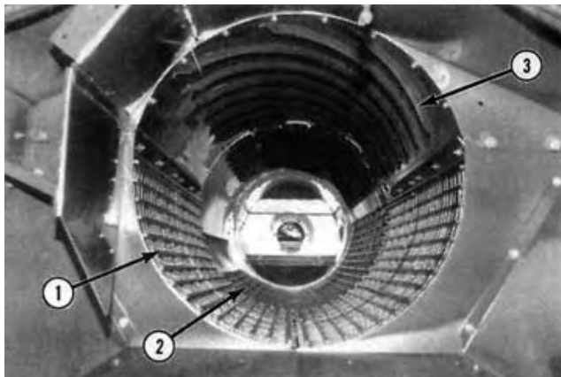
FIGURE 3. Rotor Housing: (1) Threshing Concaves, (2) Separating Concaves, (3) Vanes.
