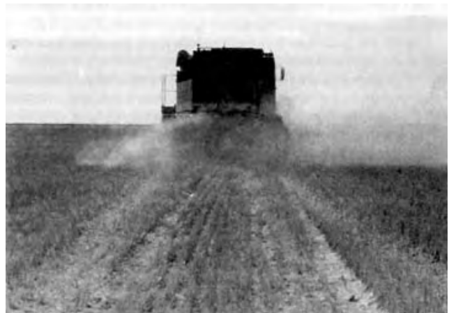
FIGURE 17. Uneven Straw Chopper Discharge.
