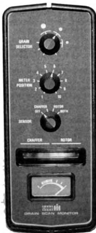
FIGURE 16. Loss Monitor Console.
