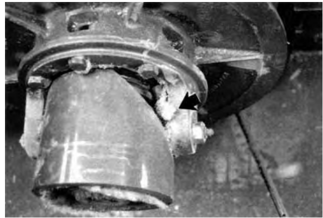
FIGURE 20. Debris in Torque-Sensing Hub.
