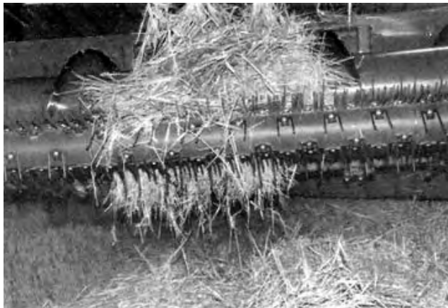
FIGURE 11. Plugging at the Pickup Stripper.
