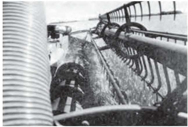
FIGURE 5. Air Providing Smooth Feeding in Short Crop.
