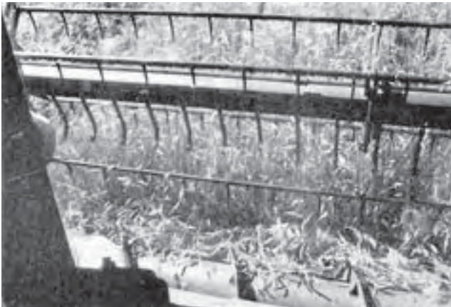
FIGURE 4. Smooth Crop Flow Along Table Auger.
