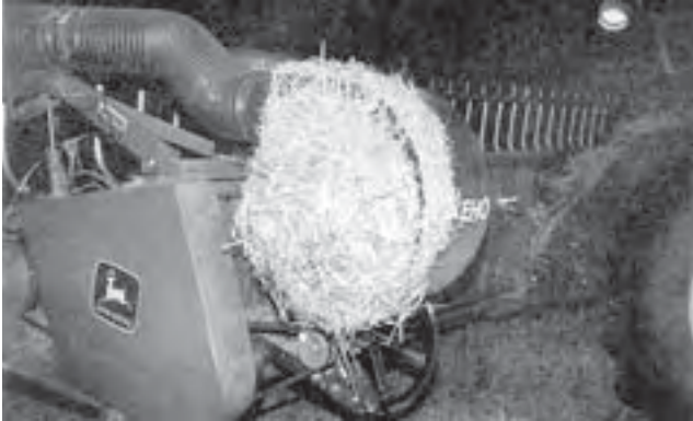
FIGURE 4. Straw and Chaff on the Fan Inlet.
