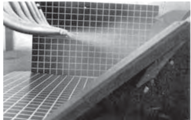
FIGURE 3. Side View of the Nozzle Discharge Pattern.
