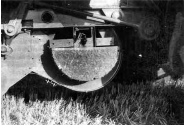
FIGURE 12. Chaff Blocking the Cleaning Fan Intake Screen.
