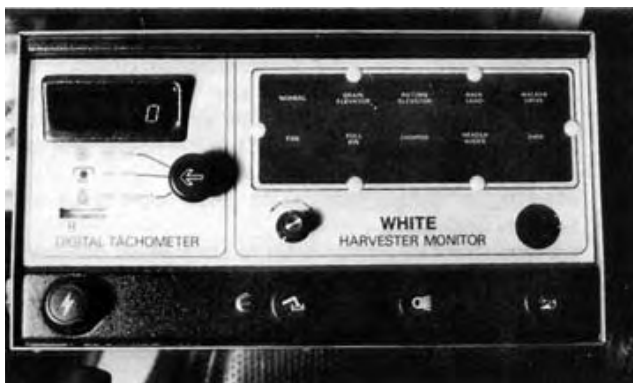
FIGURE 4. Harvester Monitor and Control Switches.
