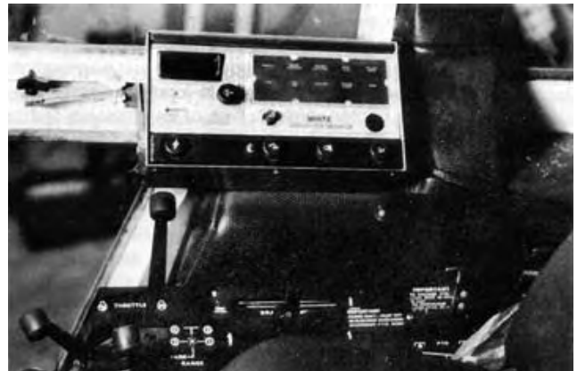
FIGURE 2. Harvester Monitor Installed in Tractor.
