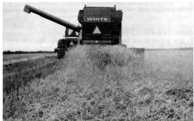
FIGURE 5. Spreading of Chopped Straw.
