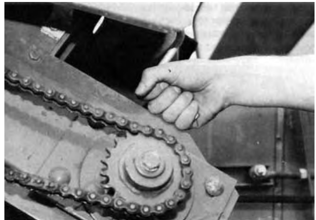
FIGURE 7. Pickup Drive Variable Speed Control.
