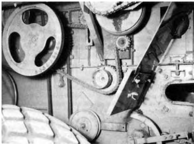
FIGURE 9. Cylinder Speed Adjustments.
