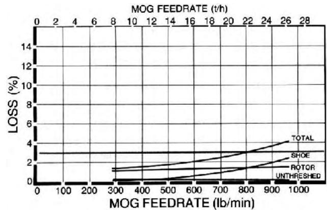
FIGURE 3. Grain Loss in Columbus Wheat.
