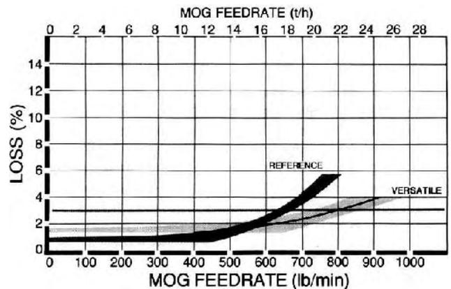
**FIGURE 6.** Total Grain Loss in Columbus Wheat.
