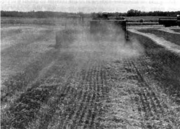
FIGURE 10. Typical Straw Spread Pattern.
