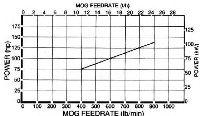
FIGURE 14. Power Requirement in Columbus Wheat.
