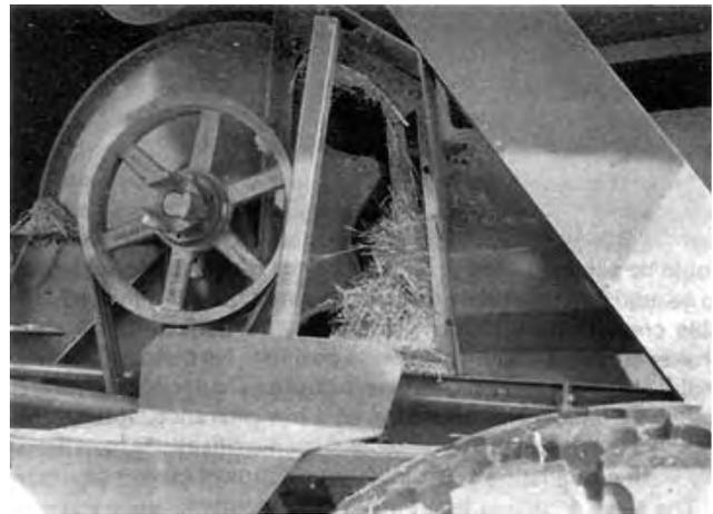
FIGURE 8. Plugging between the Cylinder and Rotor.
