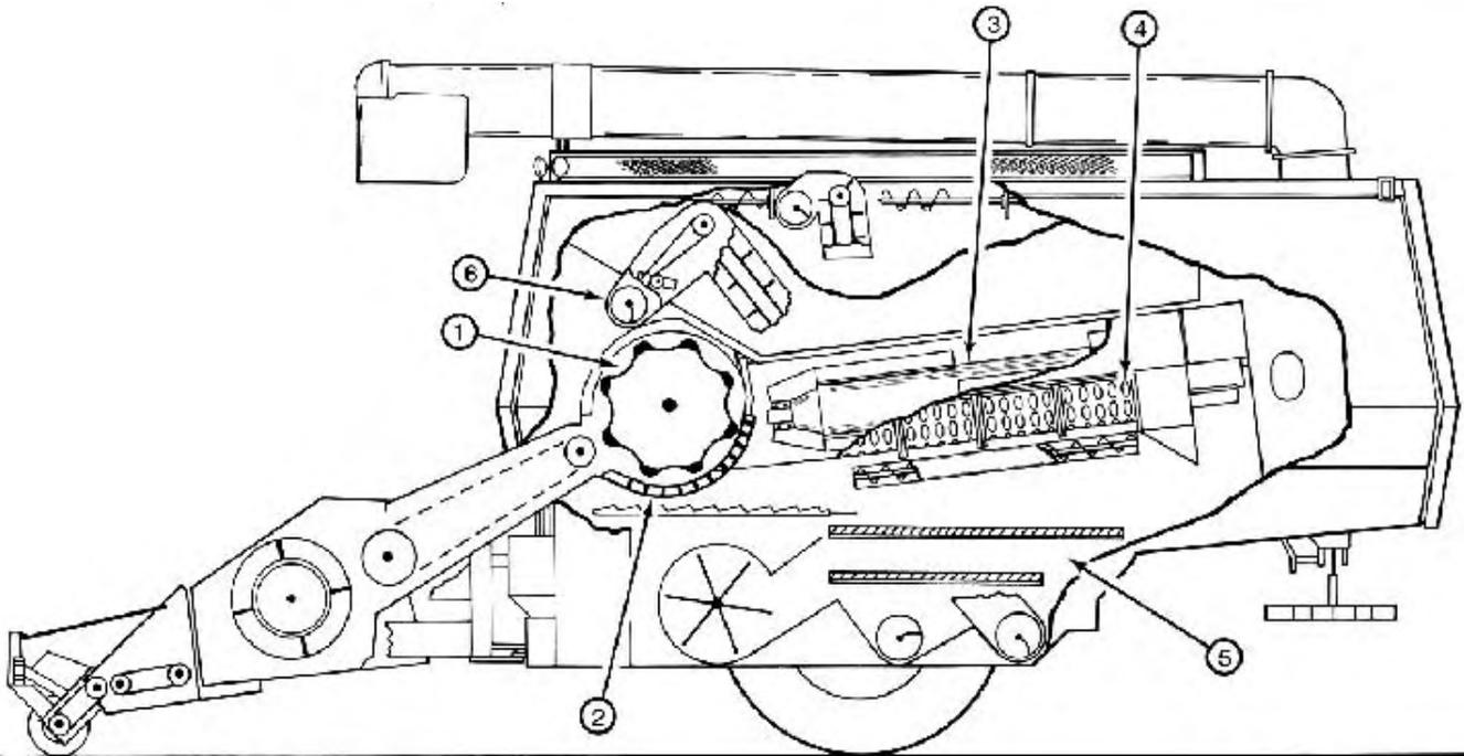
FIGURE 1. Versatile Trans-Axial 2000: (1) Cylinder, (2) Concave, (3) Separating Rotors, (4) Rotor Grates, (5) Cleaning Shoes, (6) Tailings Return.
