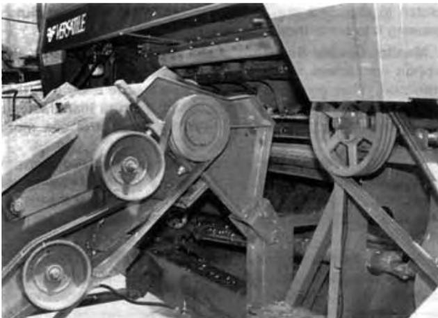
FIGURE 12. Feeder House Tilted Forward.
