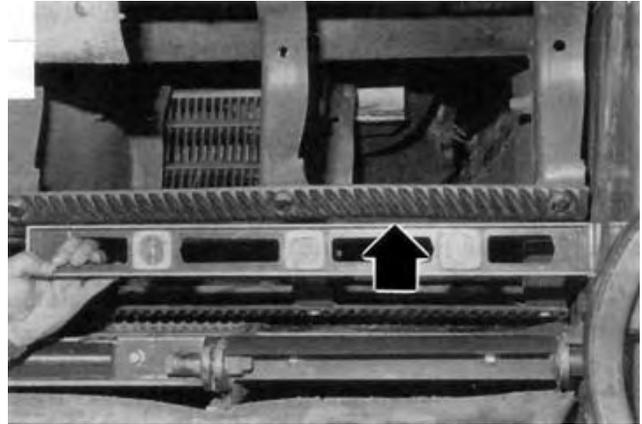
FIGURE 15. Bent Rasp Bar and Support Hub.
