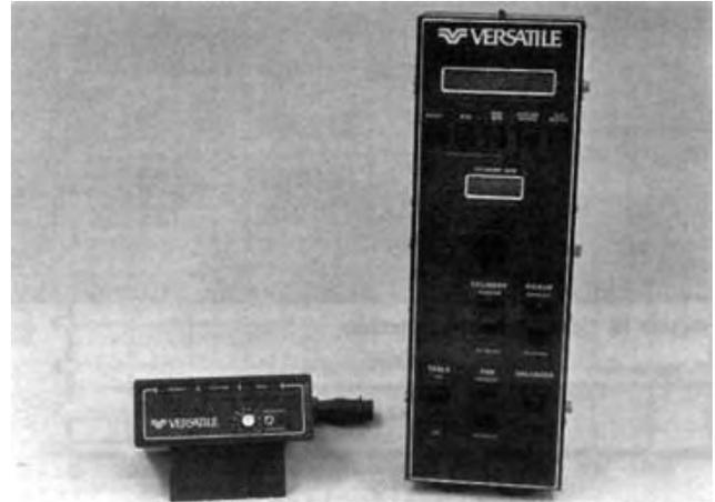
FIGURE 11. Combine Control Box and Grain Loss Monitor.
