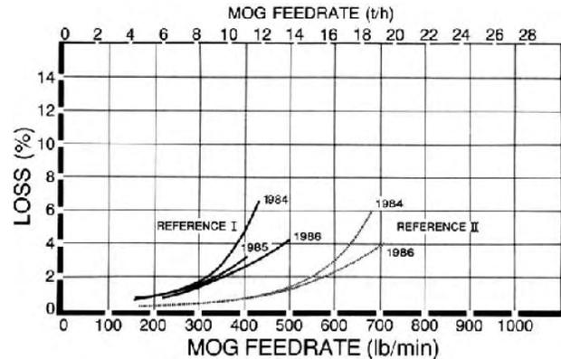
FIGURE 18. Total Grain Loss for the PAMI Reference Combines in Wheat.
