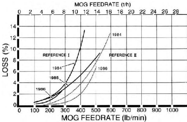
FIGURE 17. Total Grain Loss for the PAMI Reference Combines in Barley.
