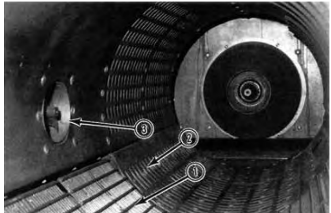
FIGURE 2. Rotor: (1) Intake Section, (2) Threshing Section, (3) Separating Section. FIGURE 3. (1) Threshing Concaves, (2) Separating Concaves, (3) Tailings Return.
