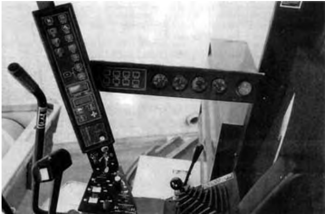
FIGURE 16. Instrument Bars and Lower Right Controls.
