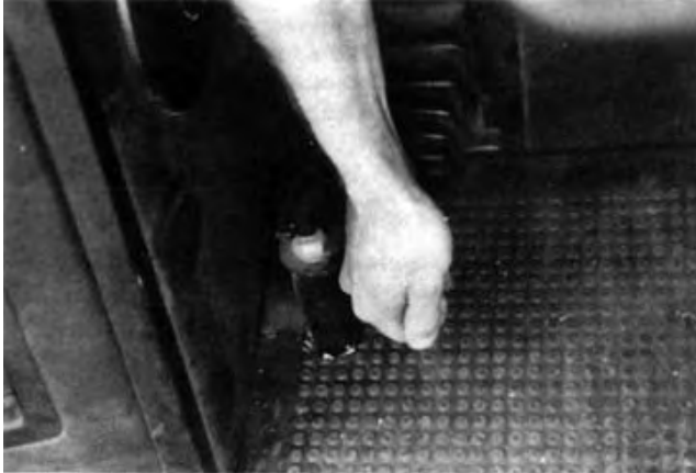
FIGURE 16. Pinch Point Between Brake Lever and Header Reverser.
