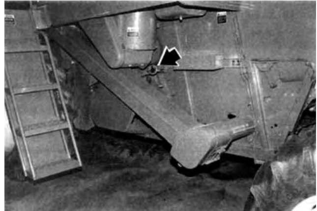
FIGURE 17. Fan Speed Adjustment and Tailings Return Elevator Sump.
