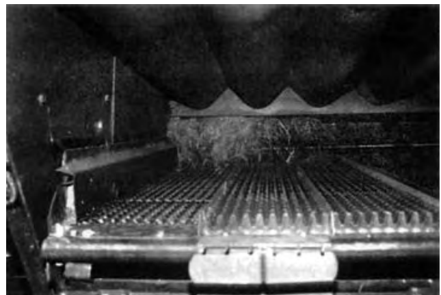
FIGURE 11. Flax Straw Wrapped on Outer Shoe Supply Augers.
