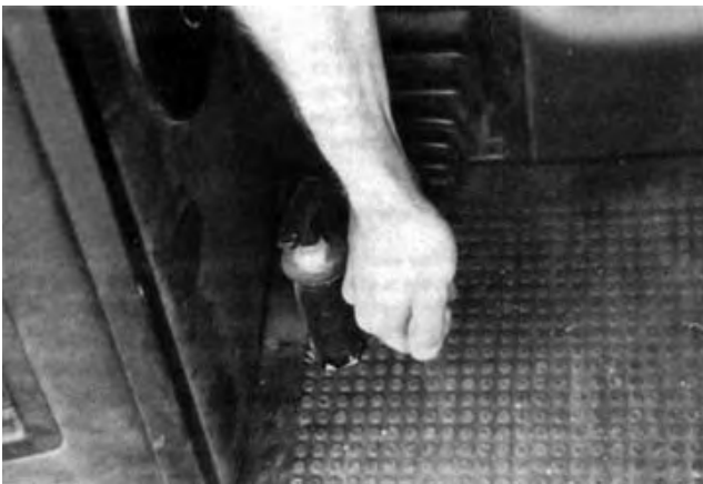
FIGURE 18. Pinch Point Between Park Brake Lever and Header Reverser.
