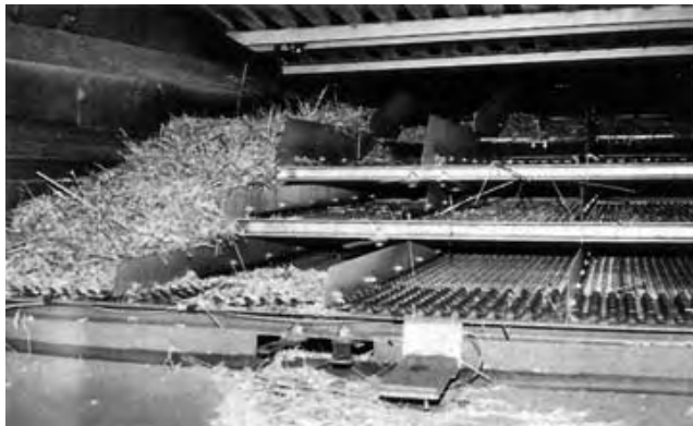
FIGURE 10. Overloading of the Left Section of the Shoe.
