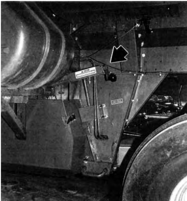
FIGURE 23. Fan Speed Control.
