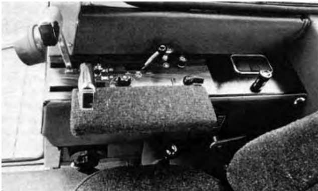
FIGURE 3. Control Console to the Right of the Operator.
