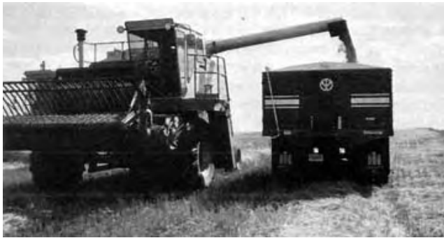
FIGURE 7. Unloading with Spout Modified by the Machinery Institute.
