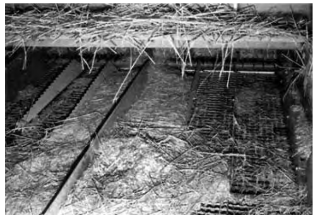
FIGURE 22. Over Loading of the Center of the Shoe.
