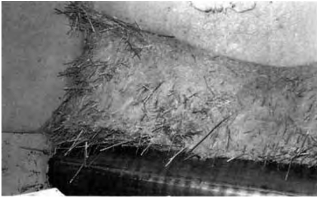
FIGURE 8. Bridging Between Feed Roll and Straw Hood Baffle.
