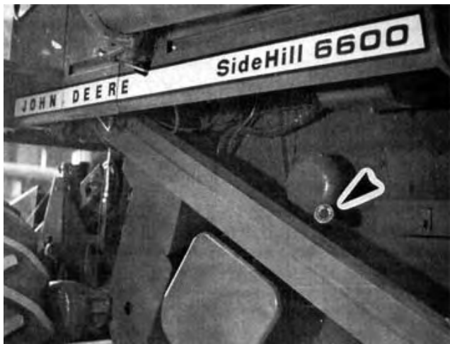
Figure 7. Fan Adjustments on the JD 6600.
