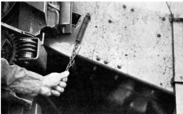
Figure 5. Stone Trap Access on the IH 914.
