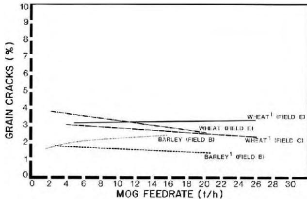
FIGURE 14. Grain Damage (Side by Side Double Windrows).
