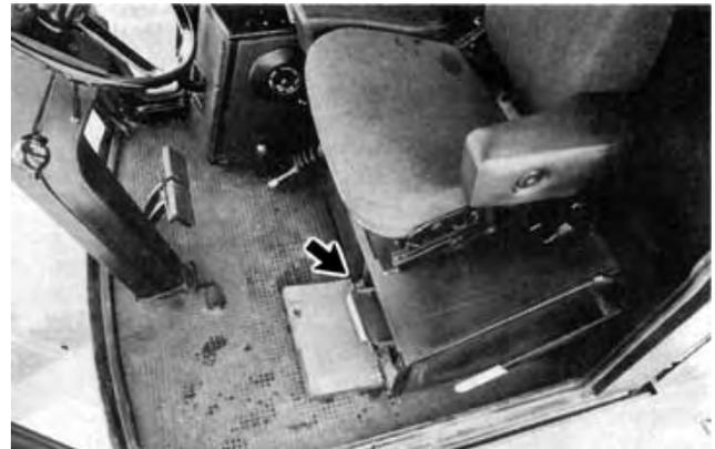
FIGURE 8. Return Tailings Inspection Port.
