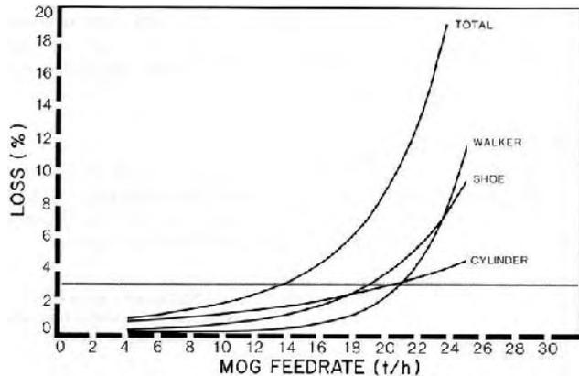
FIGURE 11. Grain Loss in Neepawa Wheat (Field C - Double Windrows).
