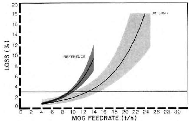
FIGURE 17. Total Grain Loss in Neepawa Wheat (Field C - Double Windrows).
