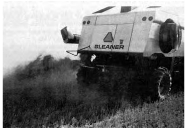
FIGURE 7. Straw Spreader Operation.
