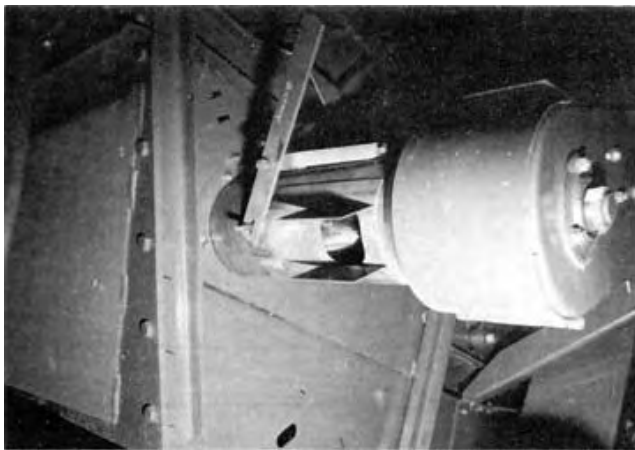
FIGURE 14. Tailings Sampling Mechanism Installed by PAMI.
