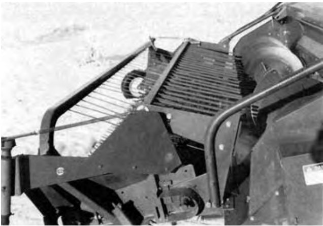
FIGURE 5. Pickup with Windguard and Crop Deflector.
