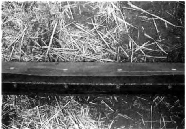
FIGURE 10. Deformed Front Panel Stripper.
