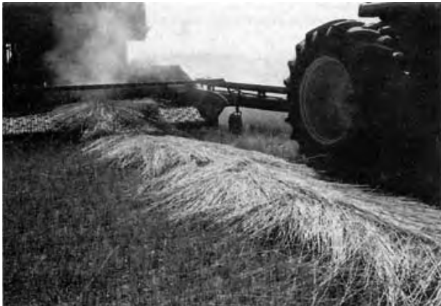
FIGURE 3. Excessive Dust at Feeder Entrance.
