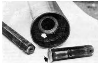
FIGURE 8. Broken Smooth Feedroll.
