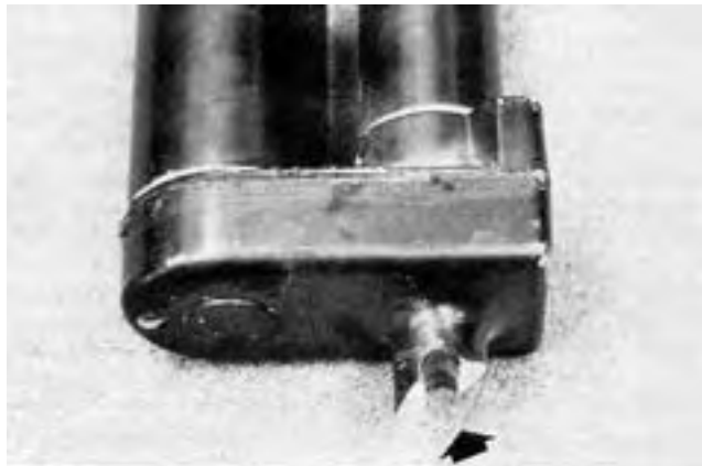
FIGURE 9. Broken Electric Actuator.
