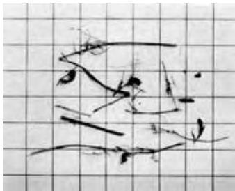
FIGURE 10. Distribution of Particle Lengths (20 mm grid).
