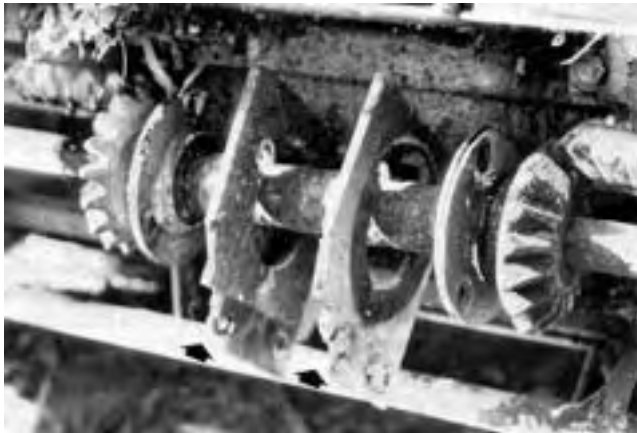
FIGURE 8. Broken Bearing Supports.
