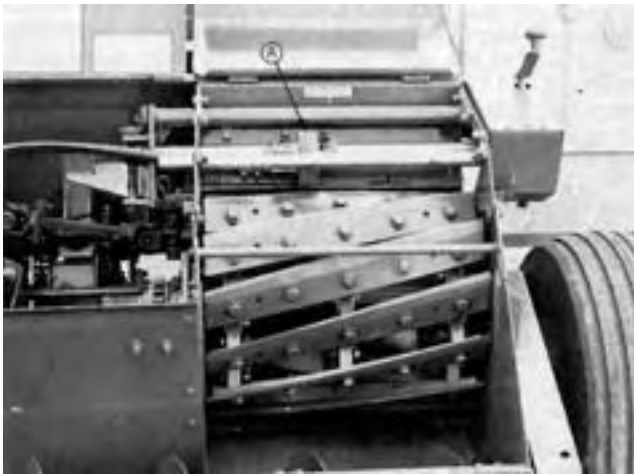
FIGURE 5. Cutterhead Knife Sharpening: (A) Cylindrical Stone.
