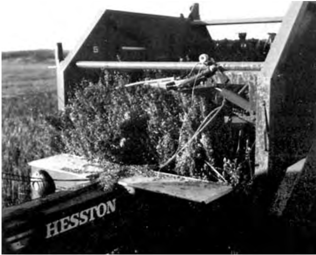
FIGURE 7. Accumulation of Hay on Front Bale Forming Grid in Heavy Windrows.
