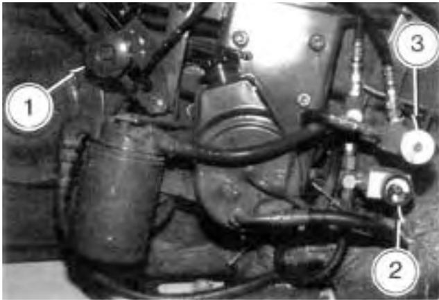
**FIGURE 6.** Bale Settings: (1) Bale Size Control Knob, (2) Twine Wrap Control Valve, (3) Net Wrap Control Valve.
