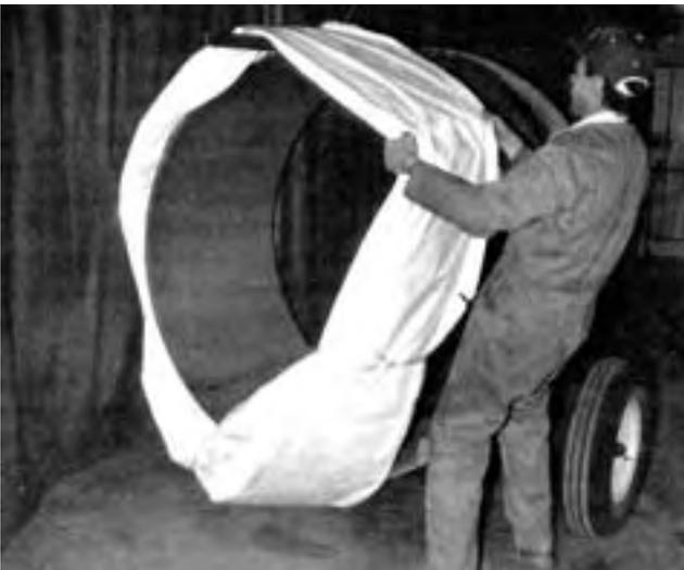
FIGURE 4. Installing Folded Poly Tubing onto the Drum.
