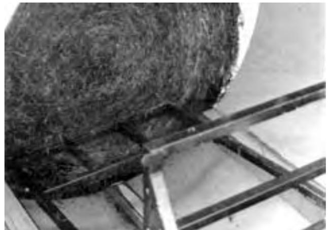
FIGURE 6. Bale Wedged Against Drop Extension Rail.
