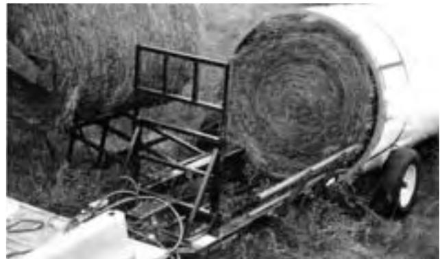
FIGURE 2. Bale from Expanding Chamber Baler being Set onto the Ramp.
