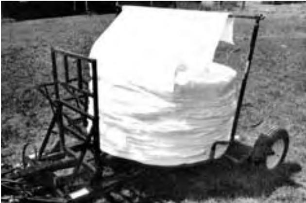
FIGURE 3. Installing Poly Tubing from Roll onto Drum.
