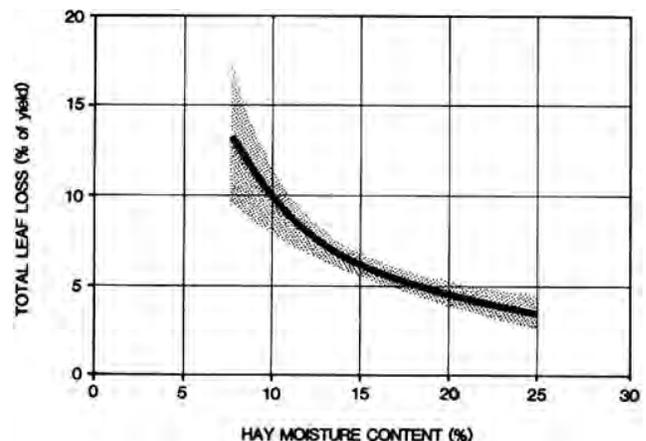
FIGURE 3. Typical Round Baler Leaf and Stem Loss in Mixed Alfalfa, Crested Wheatgrass and Bromegrass.
