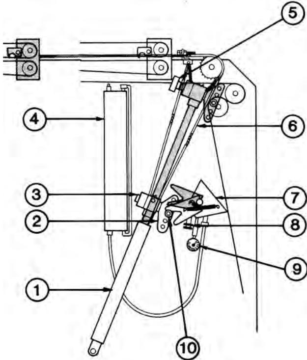
**FIGURE 6.** Total Density Control System Components: (1) Density Cylinder, (2) Trip Arm, (3) Magnet, (4) Reservoir, (5) Magnetic Sensor, (6) Loading Chain, (7) Valve Trip Mechanism, (8) Adjustable Relief Valve, (9) Pressure Gauge, (10) Trigger.
