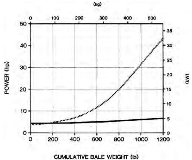
FIGURE 7. Power Consumption During Bale Formation in Alfalfa Bromegrass.
