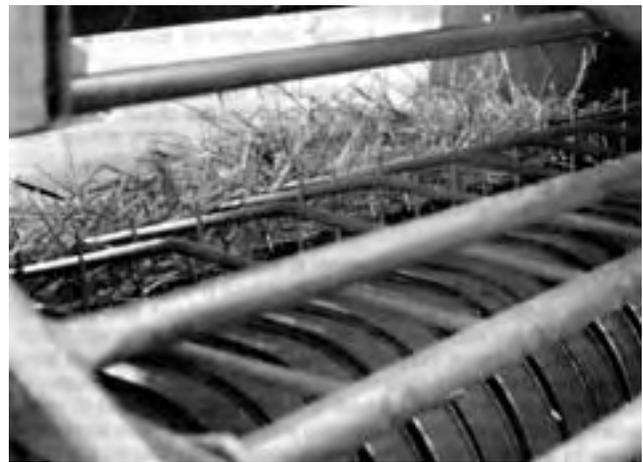
FIGURE 6. Material Caught Between Pickup and Forming Platform.
