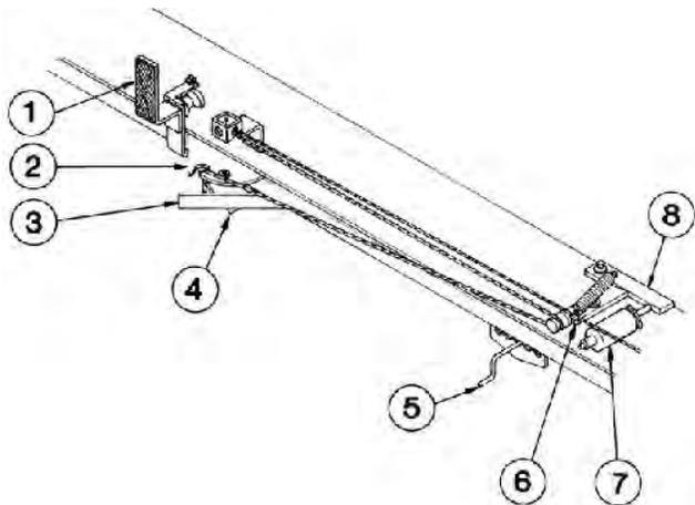
FIGURE 5. Twine Tying Mechanism: (1) Reflector, (2) Twine Guide, (3) Twine Holder, (4) Twine Knife, (5) Twine Adjustment Rod, (6) Twine Arm, (7) Solenoid, (8) Trip Lever.
