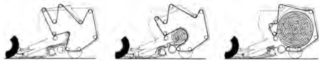
FIGURE 5. Stages of Bale Formation: (Left) Starting Bale, (Centre) Partially Completed Bale, (Right) Completed Bale.
