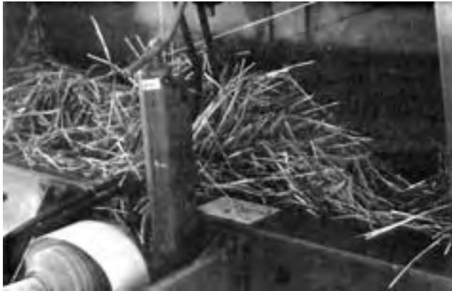
FIGURE 9. Dry Straw Piled On the Pickup Windguard Due to Backfeeding.
