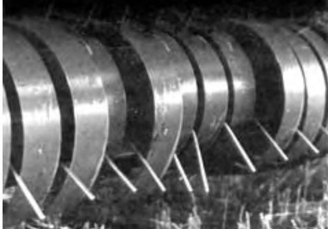
FIGURE 10. Damaged Pickup.
