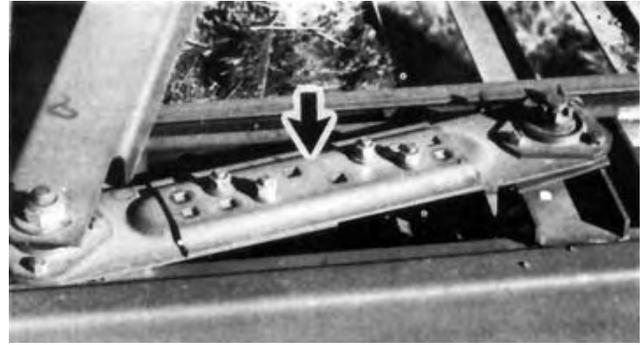
FIGURE 6. Feeder Sled Link Adjustment.
