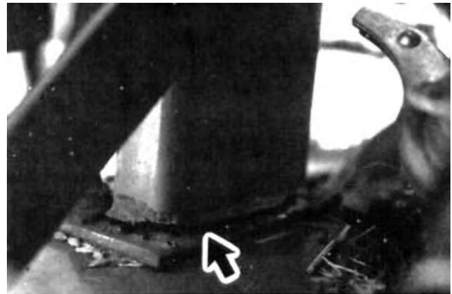
FIGURE 9. Broken Knotter Mounting Frame.
