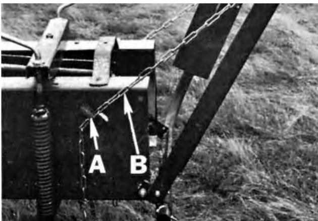
FIGURE 6. Bale Chute in Transport Position: (A) Hook, (B) Link.
