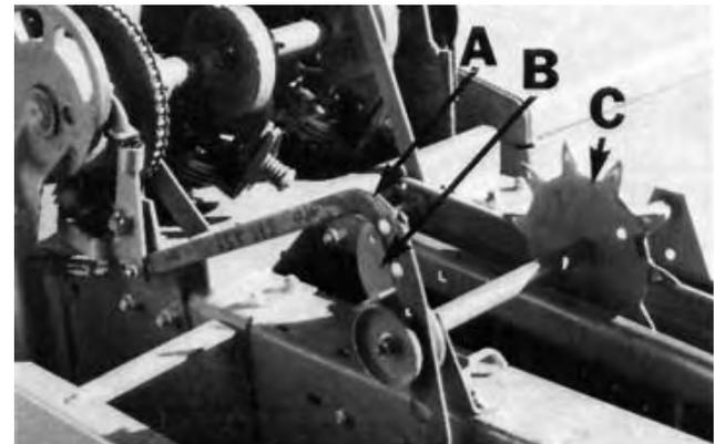
FIGURE 3. Bale Length Adjustment: (A) Metering Arm, (B) Adjustable Stop, (C) Metering Wheel.
