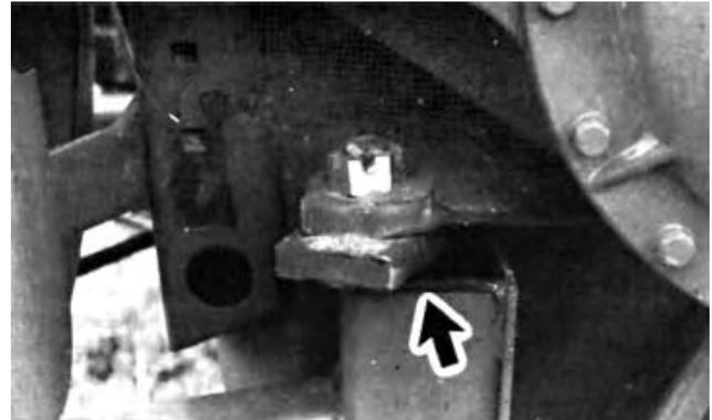
FIGURE 8. Broken Hitch Weld.
