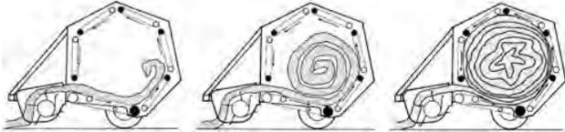
**Figure 6.** Power Consumption of the McKee 1500 During Bale Formation. Figure 6. Stages of Bale Formation. (Left) Bale Core, (Centre) Half Completed Bale, (Right) Completed Bale.
