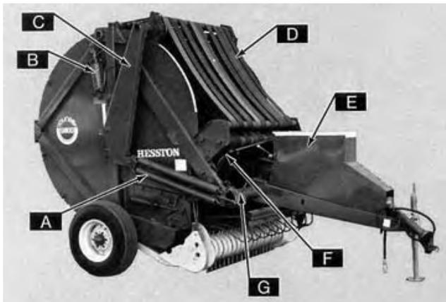
Figure 2. Front view of Hesston 5800 Rounder. Identification of Components: (A) Tension Spring, (B) Gate Cylinder, (C) Tension Arm, (D) Forming Belts, (E) Twine Box, (F) Twine Cutter, (G) Pickup Transport Lever.
