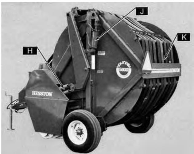
Figure 3. Rear View of Hesston 5800 Rounder. Identification of Components: (H) Tension Springs, (J) Gate Cylinder, (K) Forming Belts.
