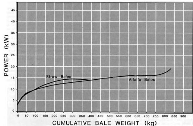
**Figure 5.** Power Consumption of the Hesston 5800 During Bale Formation.
