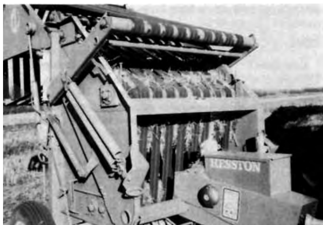
FIGURE 6. Material Build Up Between Belts.
