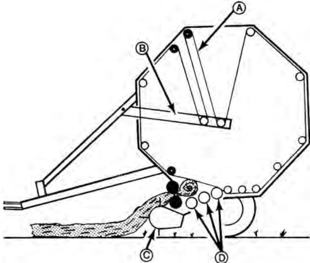
FIGURE 1. Massey-Ferguson MF 560 Balers: (A) Bale Forming Belts, (B) Tension Arm, (C) Pickup, (D) Platform Rollers.
