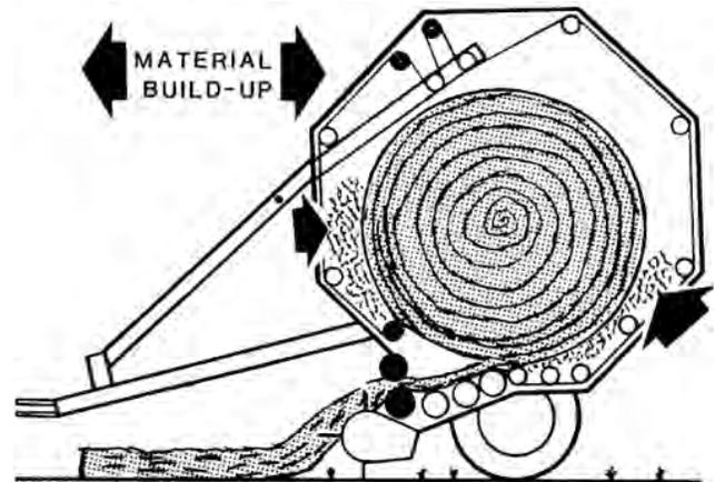
FIGURE 8. Hay Buildup Between Belts.
